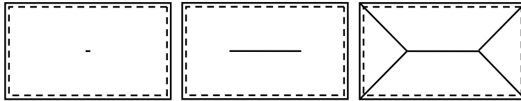
Figure 2.23 Illustration of how a plastic hinge is formed in the centre of a simply supported rectangular slab subjected to uniformly distributed load and how the yield line develops towards the corners.
